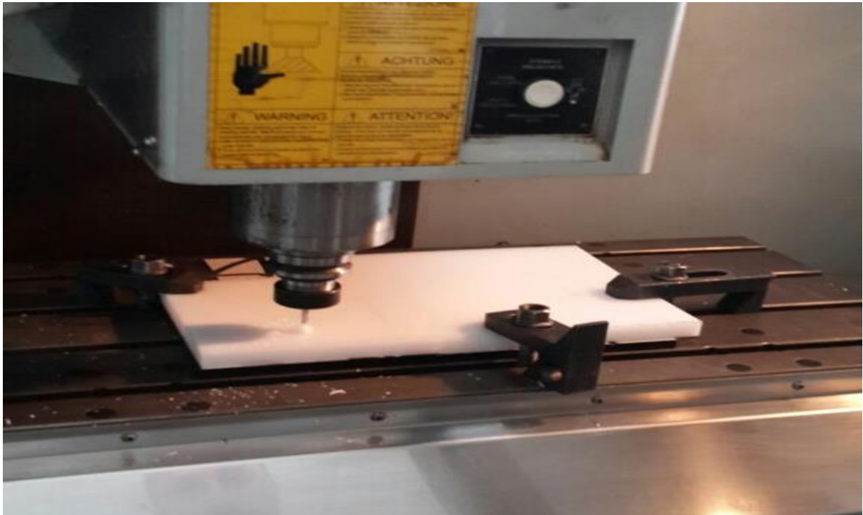
Figure 4. 4 Processing of Thermoplastic Material with Using CNC Machine.
