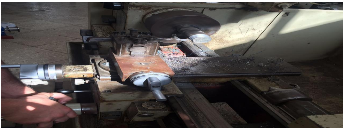
Figure 4. 16 Steel Rod Machining in Lathe
